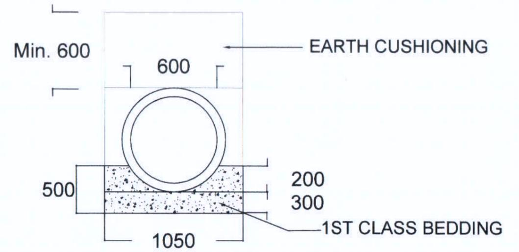
CROSS SECTION OF HUME PIPE CULVERT
