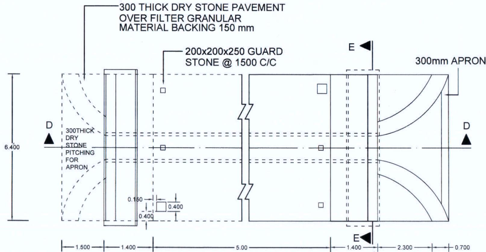
**PLAN OF 1000mm DIA SINGLE ROW CULVERT**
