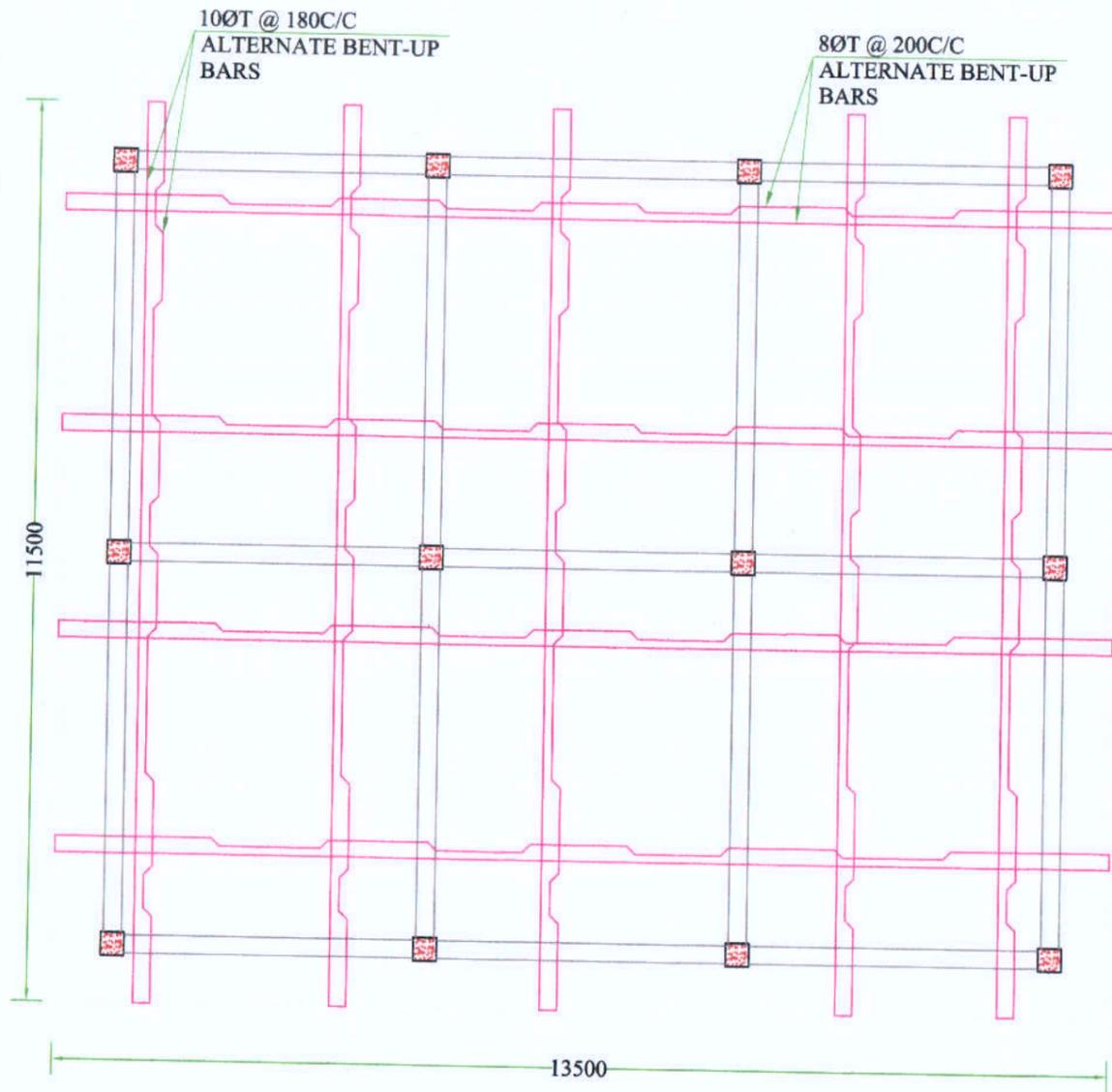
**DETAIL OF ROOF SLAB
